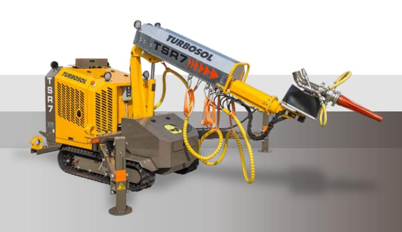
TSR 7: crawler equipment designed for shotcrete applications in jobsites with difficult access and tunnels.
